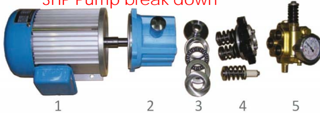
3HP Pump break down
